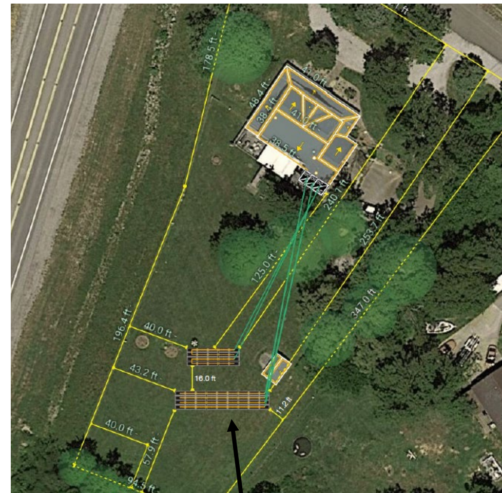
Two Proposed Ground Mount Solar Arrays Totaling 1,500 sq. ft.
